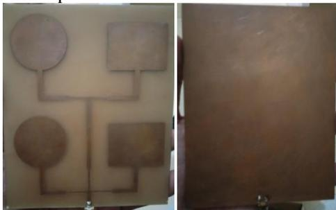
**Gambar 12** Antena Array Mikrostrip Patch Square-Circular Bahan Tembaga
