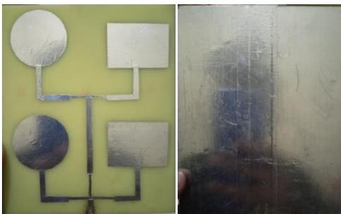
**Gambar 13** Antena Array Mikrostrip Patch Square-Circular Bahan Aluminium
